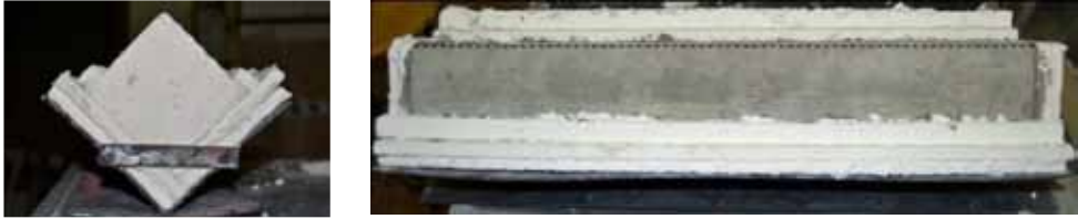
Figure 6 - Typical specimen placed on the saddle-like support and ready to be introduced into the furnace: transverse and lateral views.
