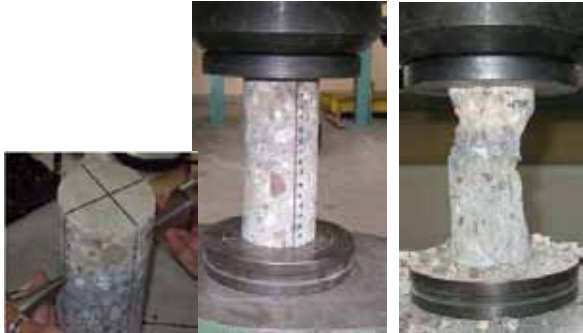
Figure 11 – Cores extracted from HPC before and after being tested in compression.
