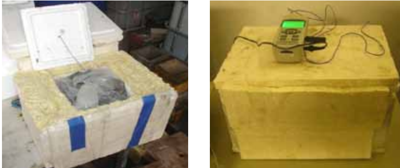
Figure 10 – Insulated box for semi-adiabatic curing conditions used for temperature measurements of the RAC mixtures.
