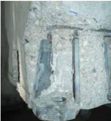
Figure 8 - Weakened shoes bolted sockets: (a) hysteretic cycles; and (b) broken shoe bar weld and details of the anchoring device.
