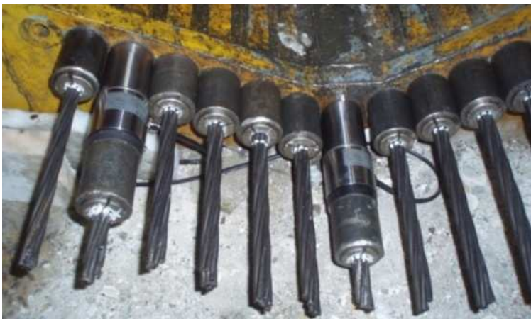
Figure 4 – Load cells mounted on two pre-stressing strands.
